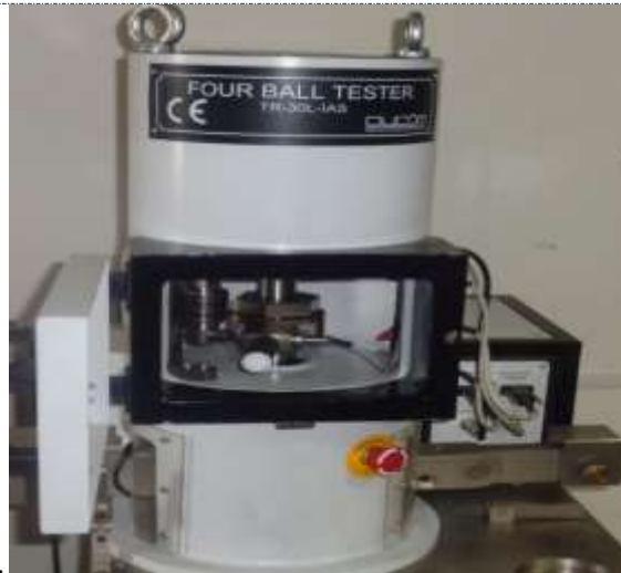
Fig.4: Four ball tester mfg.by Ducom,Bangalor,India
